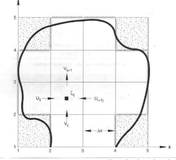
Figure 5-19 Discretization grid for 2-D circulation model. Slingerland, Harbaugh, and Furlong (1994)
